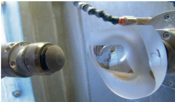
Fig. 42. Torus fabricated by Precession process [228].
