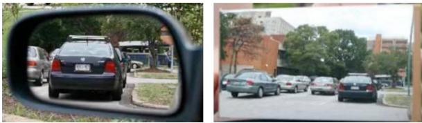
Fig. 6. Left image is from a flat driver-side mirror, and right one is from a freeform mirror [165].
