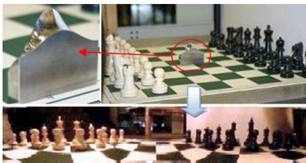
Fig. 8. Freeform mirror (above) for panoramic image (below) [82].
