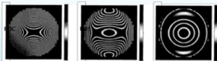
The surface shapes that resulted in the operational recovery of the optical wavefront for the science instruments on the Hubble Space Telescope. The aspheres are uncompen-sated and at the center of curvature.
