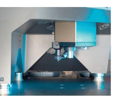
Micro-motors, micro-switches and precision components are showing up in more and more areas of our lives. Their reliability depends on their quality which is defined by measuring. With its intricate parts, micro-system technology is the challenge facing touch or optical measuring. Extremely small dimensions and different forces exist here; other principles apply. With the F25, Carl Zeiss has developed a coordinate measuring machine capable of measuring micro-system components.
